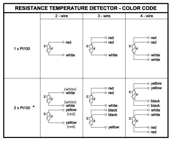
\* Colour in brackets for Type MW08 and MW08-Ex
